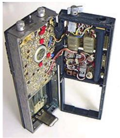
This was the one all the hams wanted because of its selectable high-low power. Motorola decided to develop and market this model for the new VHF marine band (156 MHz) which replaced in the 1970s the old shortwave marine band.
